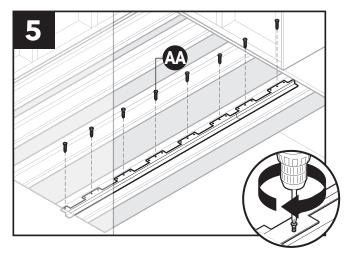
Secure main bracket to floor joist with one #8 flat-head Phillips screw (AA) per tab. Only **one hole** (preferably the middle hole) on each tab should be used unless circumstances make middle hole unavailable.
