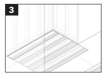
Note the linear drain location (C and D brackets will be installed in the back opening later in installation process).
