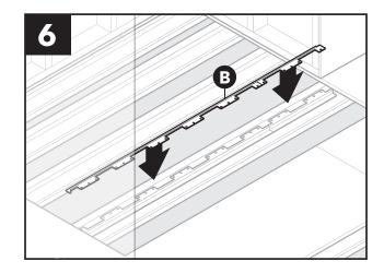
Place main bracket (B) on other side of floor joist (bracket should be flush against top and side of joist). Cut main bracket (B) to size if needed.
