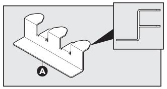
**Z brackets** (A) upper tabs will be installed under the base plate where there is a wall at the shower pan and on top of plywood at recess transition.
