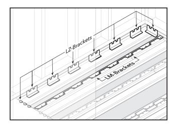
Linear Drain Bracket Placement Parallel joists.
