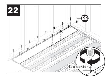
Secure plywood strip to Z-brackets and main bracket with #10 1 5/8" wood to metal self-drilling screws with wings with wings (BB). Screw down every 10-12" minimum.
