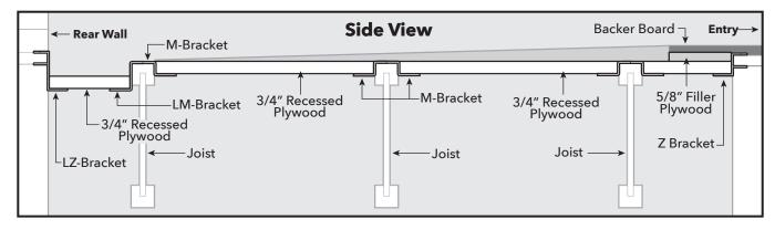
Overview of bracket and recess plywood placement (side view).
