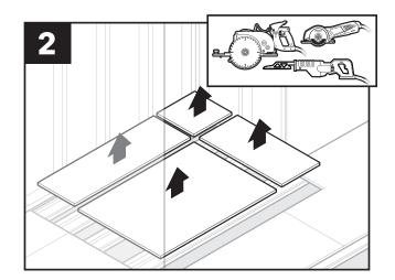
Use recommended saw to flush cut marked portions subfloor and remove.
