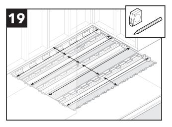
Measure distance between main brackets on floor joists and Z-brackets for length and width for plywood strips.
