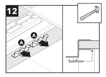
Place Z-brackets (A) into position (two per linear foot) on top of subfloor at threshold (or at the side of shower where there is no framed wall) with tabs above and below subfloor.
