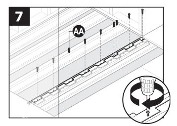
Secure main bracket to floor joist with #8 flat-head Phillips screws (AA).
