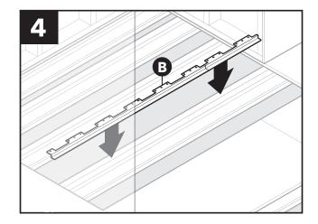
Cut main bracket (B) to size if needed. Remove any adhesive left over from the original plywood. Place main bracket (B) on one side of floor joist (bracket should be flush against top and side of joist).
