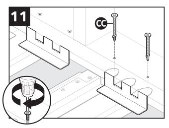
With Z-brackets (A) mounted in a level position, install #10 2 3/4" wood to metal self-drilling screws with wings (CC) through base plate and into both outer tabs of Z-brackets.
