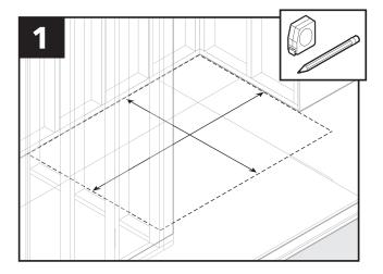
Measure and mark subfloor to be removed.
