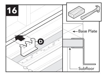
Place a LZ-bracket (D) in last opening between floor joists with tabs above and below subfloor. Use a scrap 2 x 4 during installation to keep form damaging bracket.
