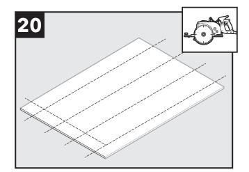
Using measurements from previous step, cut plywood strips 1/8" shorter and narrower to fit loosely into opening.
