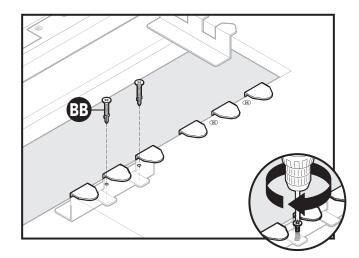
**OPTIONAL:** Secure Z-bracket by installing #10 zinc-plated Phillips flat-head reamer screws with wings (BB) through the subfloor and into the Z-bracket lower tabs.
