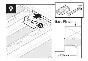
Place a Z-bracket (A) along side wall with tabs above and below subfloor. Use a scrap 2 x 4 during installation to keep from damaging bracket.
