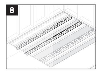
Repeat steps 4-7 for remaining floor joists and main brackets (B) except for the linear drain opening.
