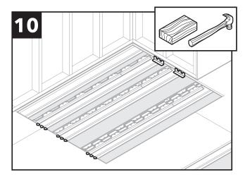
Continue placing Z-brackets along side walls (one brackets per linear foot and one bracket per opening between floor joists). Use a scrap 2 x 4 during installation to keep from damaging bracket.
