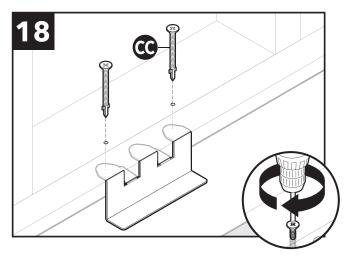
With LZ-brackets (C) mounted in a level position, install #10 2 3/4" wood to metal self-drilling screws with wings (CC) through base plate and into both outer tabs of Z-brackets.
