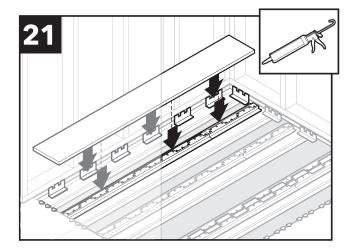
Use construction adhesive for plywood and brackets. Place first plywood strip into position on brackets.
