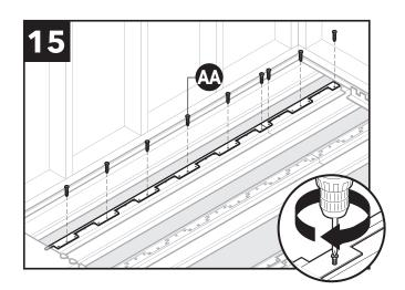
Secure LM-bracket (C) to floor joist with one #8 flat-head Phillips screw (AA) per tab. Only **one hole** (preferably the middle hole) on each tab should be used unless circumstances make middle hole unavailable.
