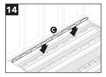
Cut LM-brackets (C) to size if needed. Remove any adhesive left over from the original plywood. Place LM-bracket (C) on inside of last floor joist (bracket should be flush against top and side of joist).
