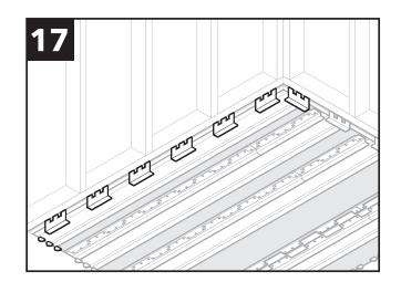
Continue placing LZ-brackets (D) along rear wall and side of last front opening (one bracket per linear foot). Use a scrap 2 x 4 during installation to keep form damaging bracket.
