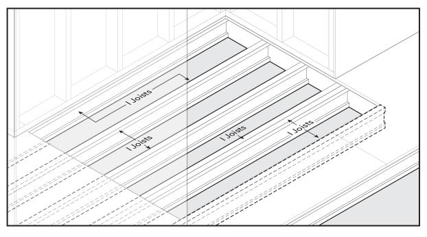
When joists are parallel to the shower entry, the transition to recessed floor needs to be placed on the front (the edge of a joist adjacent to the recessed part) edge of floor joist regardless of placement. Sometimes the recess needs to be extended past the intended shower pan. The space will be treated the same as any recessed one but filled back in with 5/8" thick plywood up to the intended shower pan.
