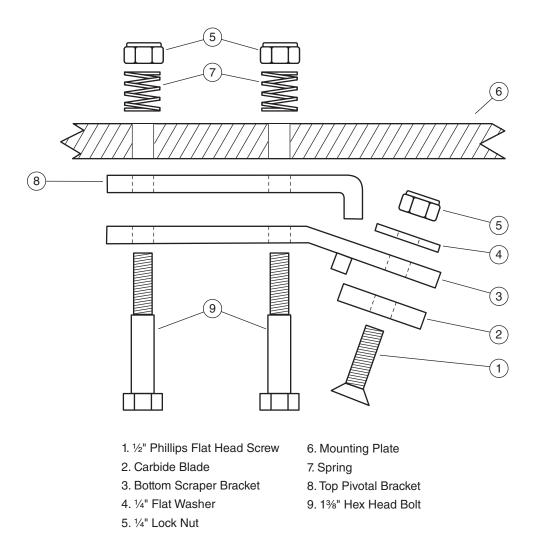
**Note:** Inspect all cutter assemblies every three (3) hours of operation and replace all worn or broken parts.
